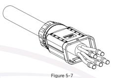
Insert the cable into the rubber core according to the line sequence, observe the perspective hole, the cable is in place, and the torque of the crimping screwdriver is 5 ± 0.1N.m.
