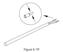
③ Fix all the wires to the terminal plug according to the assignment and tighten to a torque of 1.2+/-0.1N·m with a screwdriver.
