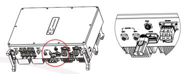
Figure 5-10 Monitoring device installation
