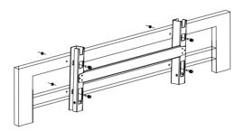
Figure 4-6 Fixing the bracket
