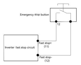
Figure 5-28 Fast stop connection diagram
