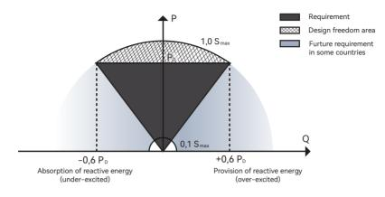
The inverter provides a reactive power regulation function.
