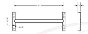
Figure 4-4 Dimensions of bracket
