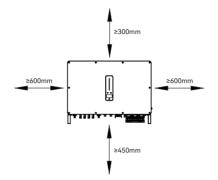
Figure 4-2A Spacing for installing an inverter
