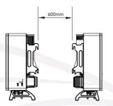
Figure 4-2C Spacing for Back to Back Installation
