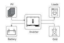
When the grid fails, power from PV and battery will supply loads connected on the back-up side (UPS).
