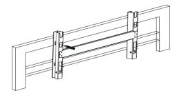
Figure 4-5 Marking hole position using installation bracket
