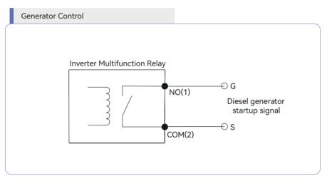
Figure 5-26 Generator Control connection diagram
