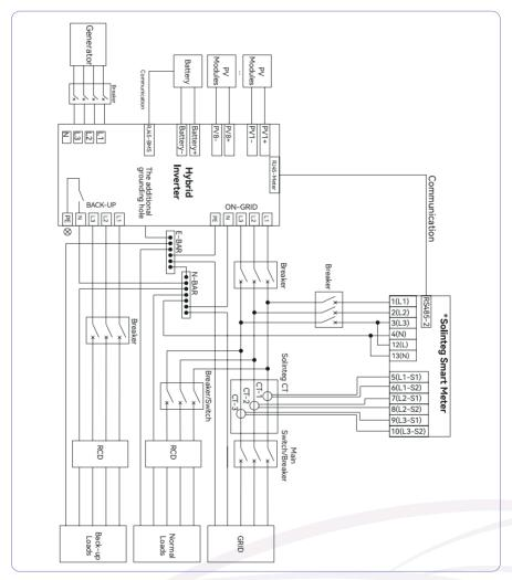
Figure 5-3 Australia wiring diagram
