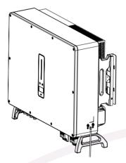
Figure 4-8 Grounding terminal connection
