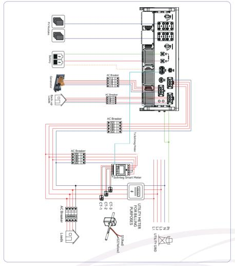
Figure 5-1 Electrical wiring diagram
