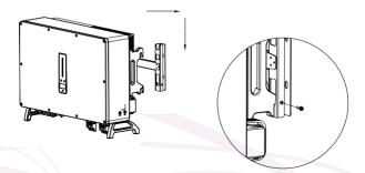
Figure 4-7 Mounting the inverter
