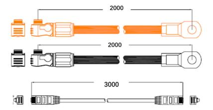
For the external cables, the length shall less than 3 meters.
