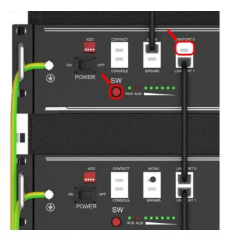
Press the red SW button of master battery to power on, all the battery LED light will be on one by one from the Master battery:
