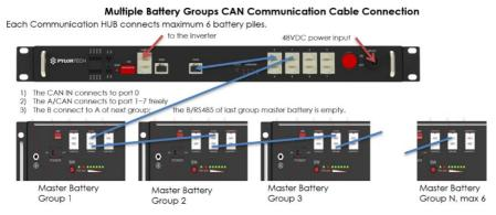
Each battery pile can configure maximum 16pcs US2000C/US3000C.
